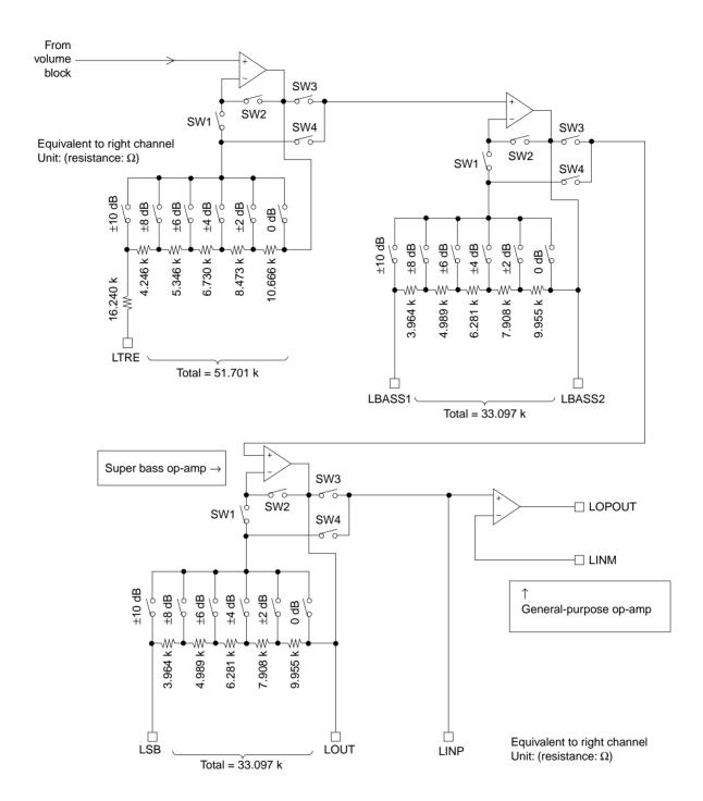
During boost, SW1 and SW3 are on, during cut, SW2 and SW4 are on, when 0 dB, 0dBSW and SW2 and SW3 are on. SW3, SW4 of super bass block are always off.
